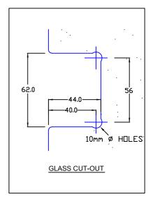
TFH1-38 and TFH1-50 Wall to Glass side mounted hinge, with two back plate options. 38mm and 50mm.
