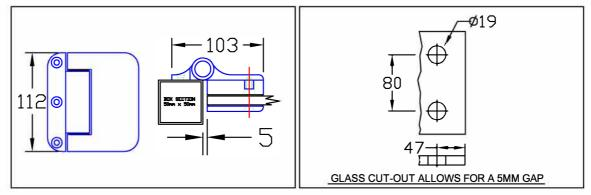
Designed for a frameless glass gate. This tension adjustable self closing hinge is designed to suit a 50mm square post to glass application and is ideally suited for use on pool gates
