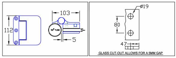
Designed for a frameless glass gate. This tension adjustable self closing hinge is designed to suit a 50mmm diameter round post to glass application and is ideally suited for use on pool gates
