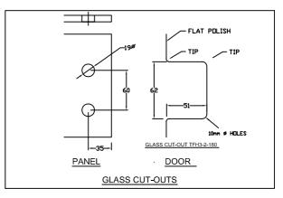
TFH3-2-180 Glass to glass hinge to mount a door to a fixed glass side panel that runs on a 180 degree plane. The hinge is secured to the panel with two holes in the glass instead of a cut-out. This results in a simpler and cheaper glass preparation. Additional advantages are better holding capabilities, and a cost effective hinge.
